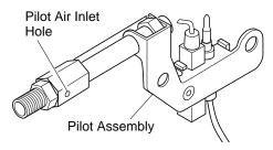
Figure 28 - Pilot Inlet Air Hole
